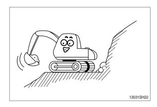
The swing on the slope can be danger of rolling over.
